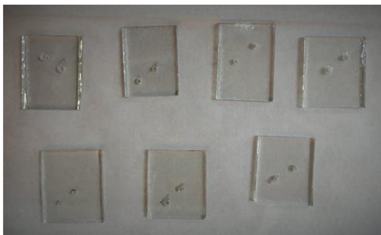
Figure 4.14. FTO-glass plates were cut into 2.5 x 2 cm pieces with two holes drilled into each piece
