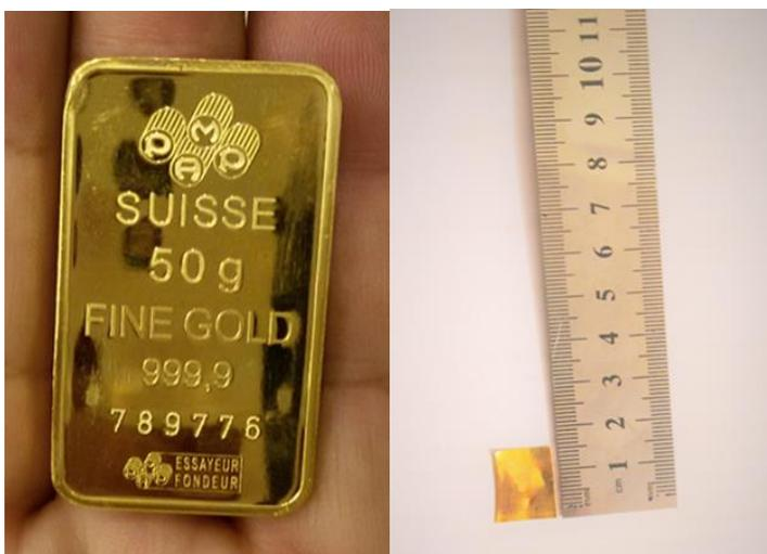
Figure 4.4. Gold target ounce from PAMP and plate target after drawing by draw machine
