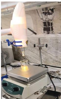
Figure 4.3. Optical emission from the laser interaction with the Au target
