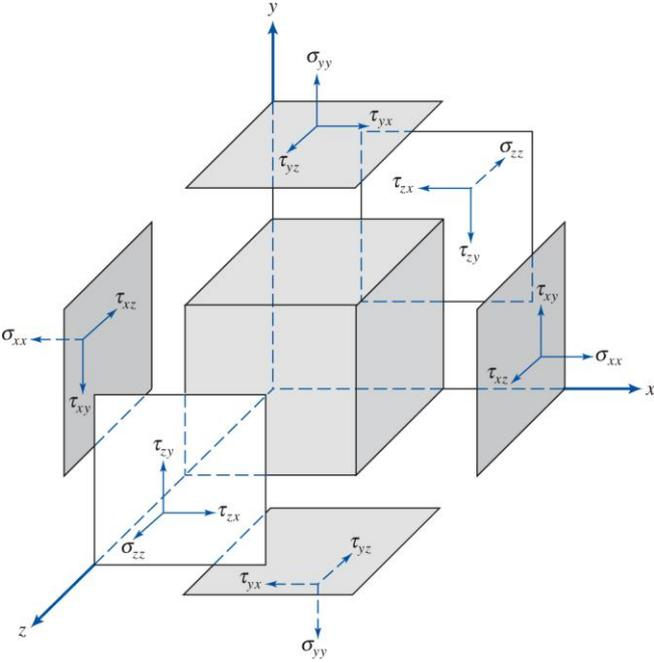
An infinite number of planes can be passed through point C, resulting an infinite number of stresses associated with that point. Fortunately state of stress at a point can be described completely by specifying the stresses acting on three mutually perpendicular planes through the point. Hence, stress at a point is specified by the nine components.
