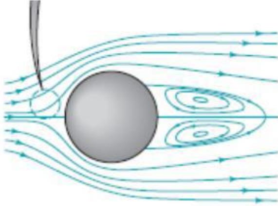
In steady flow, pathlines, streaklines, and streamlines are identical lines in the flow field.
