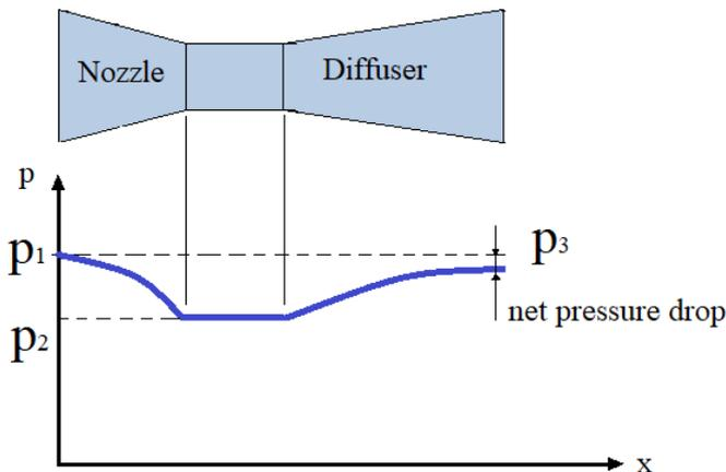
Because, we assumed the water is inviscid, the static pressure drop ( $p_1 - p_2$ ) is fully recovered in the diffuser by decreasing the fluid velocity to  $V_1$ . However, full pressure recovery would not occur in a real venturi tube. Viscous effects would produce a net pressure drop between 1 and 3.
