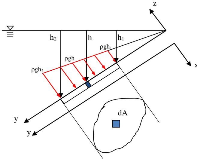
Considering the gage pressure at the free surface is zero, the infinitesimal pressure force,  $d\vec{F}$ , acting on the submerged plane surface is,
