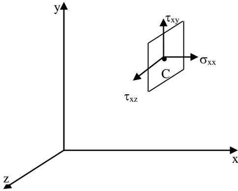
Force components on element of area  $\delta A_x$       Stress components on element of area  $\delta A_x$
