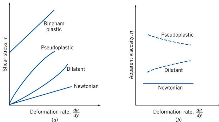
Pseudoplastic Fluid (Shear thinning): apparent viscosity decreases with increasing deformation rate.
