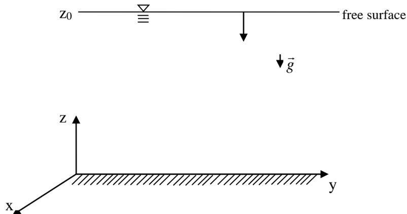
For liquids, it is often convenient to take the origin of the coordinate system at the free surface, and measure the distance as positive downward from the free surface with  $h$  measured positive downward, the
