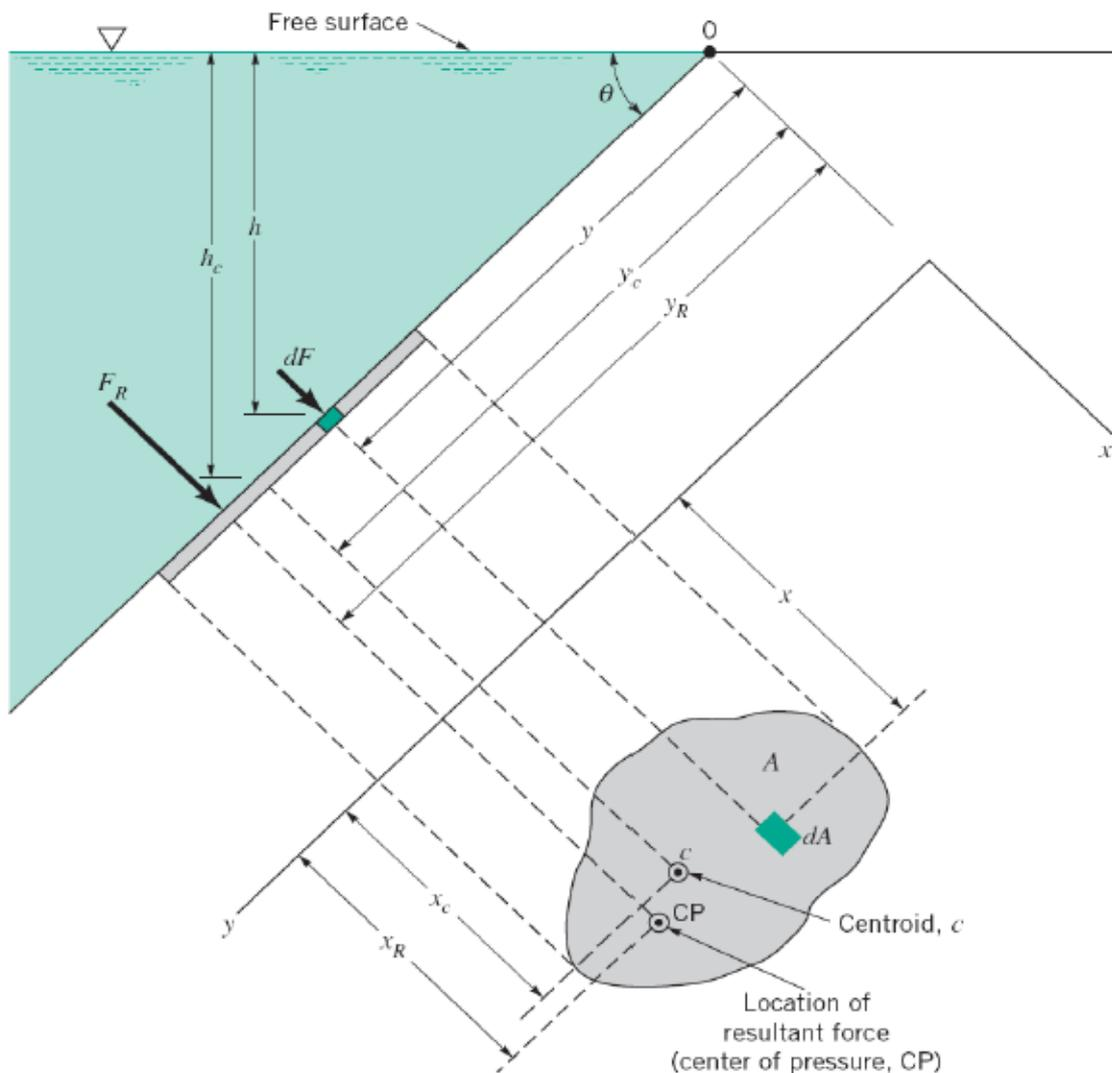
**Note:** Origin of the coordinate system is placed at the intersection of the plane of the gate and the free surface.
