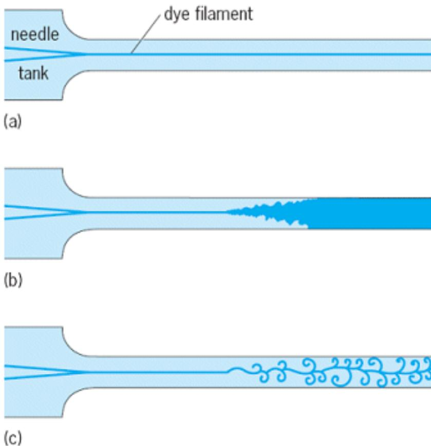
Pipe-flow transition experiment. (a) laminar flow. (b) High ReD, turbulent flow. (c) Spark photograph of turbulent flow condition. (After O. Reynolds, an experimental investigation of the circumstances which determine whether the motion of water shall be direct or sinuous and of the law of resistance in parallel channels, Phil. Trans. Roy. Soc., London, A174:935–982, 1883)
