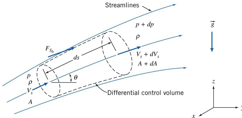
The control volume chosen is fixed in space and bounded by flow streamlines, and it is thus an element of a stream tube. The length of the control volume is  $ds$ .
