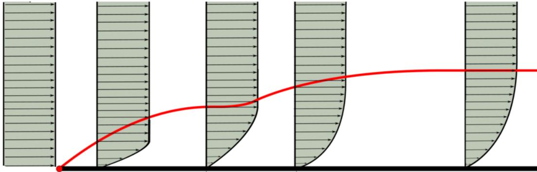
In any viscous flow, the flow in direct contact with a solid boundary has the same velocity as the boundary itself. There is no slip at the boundary.
