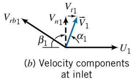
The angle of the absolute fluid velocity  $\alpha$  is measured from the normal.
