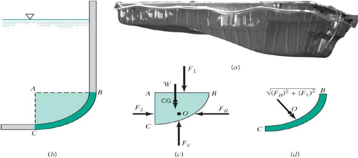
Consider the **section BC** shown in the figure above. This section has a unit length perpendicular to the plane of the paper.
