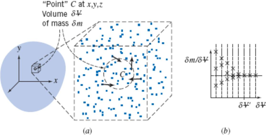
Fig. 2.1 Definition of density at a point.
