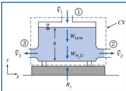
The force exerting on the control volume in the y-direction may be found by applying the momentum equation in y-direction.
