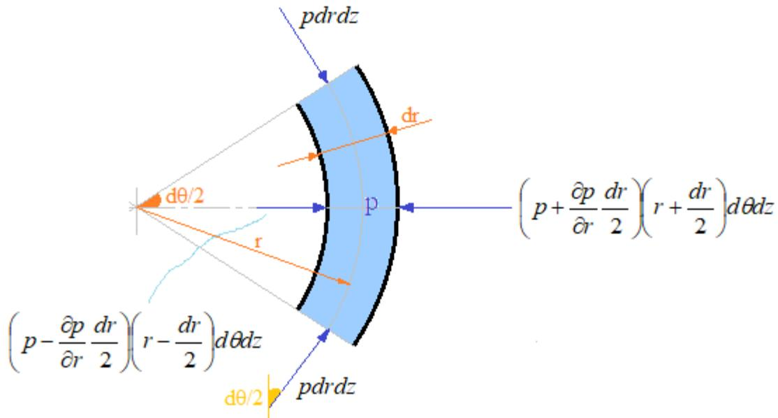
The pressure at the center of the element is P. Using a Taylor series expansion, we express forces acting in the rθ plane on the element as shown in the figure.
