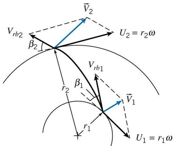
**Blade angles  $\beta$  are measured relative to the circumferential direction.**
