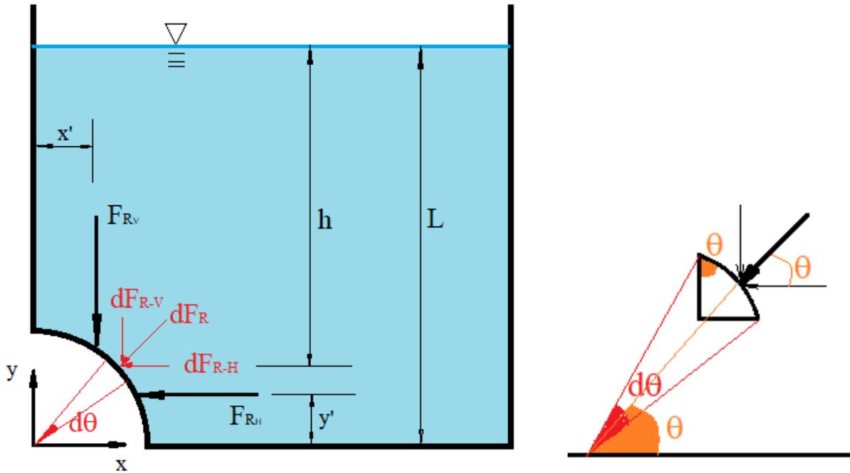
Consider the area element  $d\vec{A}$ . The resultant force acting on this area element is
