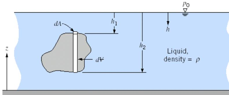
**Fig. 3.9** Immersed body in static liquid.
