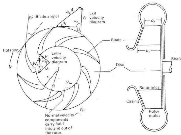
Figure 4.36 Details of flow entering and leaving a radial-flow rotor.
