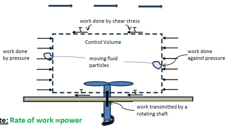
If we neglect electrical and other equivalent forms of work, three types of work might be done on or by the fluid inside the control volume as shown in the figure above
