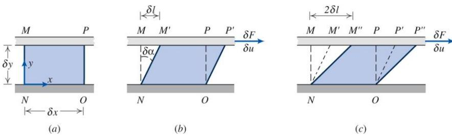
Consider the fluid element in the figure. The top of the fluid element moves faster than the bottom, so in time fluid element deform.
