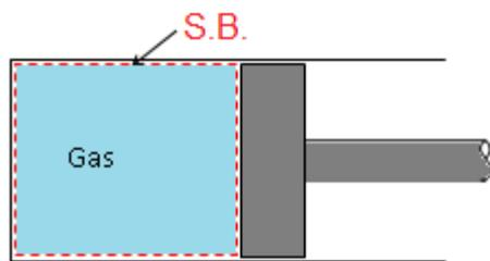
The boundaries of a system may be fixed or moveable; however, there is no mass transfer across the system boundaries; i.e. the amount of mass in the system is fixed.
