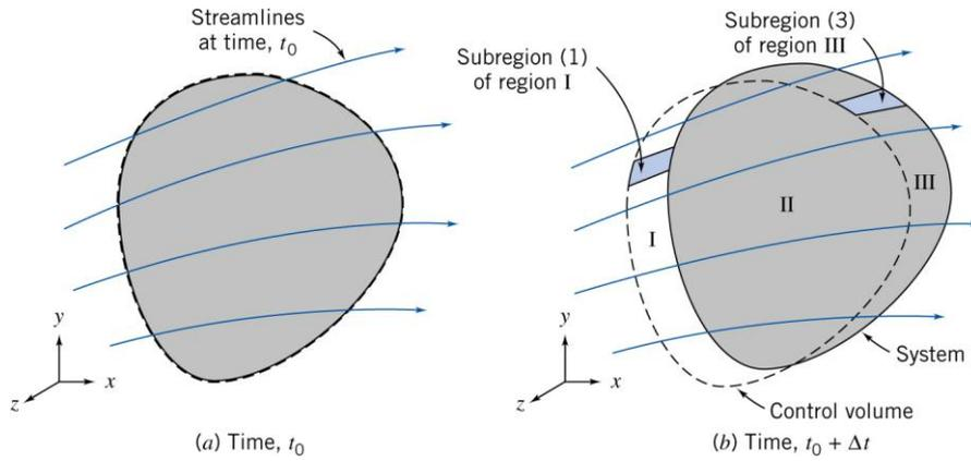
**Objective:** To relate the  $\left. \frac{dN}{dt} \right|_{\text{system}}$  to the time variations of this property (N) associated with the control volume.
