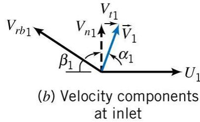
At the inlet the absolute velocity of the fluid  $\vec{V}_1$  is equal to vectoral sum of the fluid velocity with respect to blade and the tangential velocity of the rotor, i.e.
