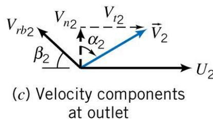
The inlet and outlet velocity polygons provide all the information required to calculate the torque or power absorbed or delivered by the impeller. The resulting values represent the performance of a turbomachine under **idealized conditions** at the design operating point; since we have assumed that all flows are uniform and that they enter and leave the rotor tangent to blades.
