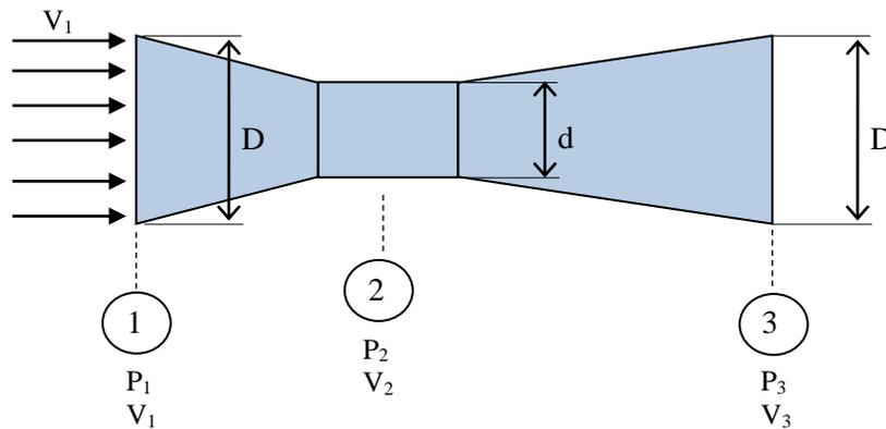
Water at  $10^\circ\text{C}$  enters the horizontal venturi tube, shown in the figure, with a uniform and steady velocity of  $2.0\text{ m/s}$  and an inlet pressure of  $150\text{ kPa}$ . Find the pressure at the throat, 2, where  $d = 3.0\text{ cm}$  and at the exit where  $D = 6.0\text{ cm}$ .
