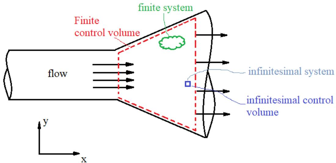
The system of point of view is related to a Lagrangian description of flow. Its advantages is that all the fundamental laws may be expressed directly in terms of a specific collection of mass.
