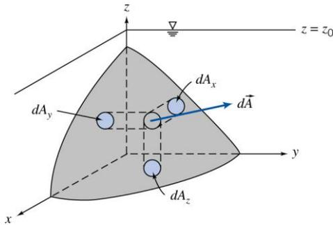
Consider the infinitesimal curved surface shown in figure. The hydrostatic force on an infinitesimal element of a curved surface,  $d\vec{A}$ , acts normal to the surface. However, the differential pressure force on each element of the surface acts in a different direction because of the surface curvature.
