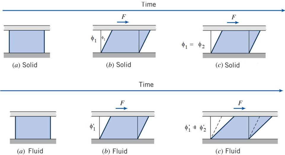
Figure 1. Solid and fluid behavior under shear stress.
