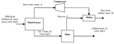
12. Several streams are mixed as shown in Figure . Calculate the flows of each stream in kg/s.
