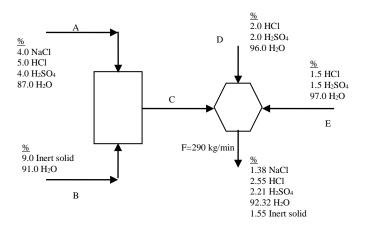
13. In the process shown in the Figure Unit I is a liquid-liquid solvent extractor and Unit II is the solvent recovery system. For the purposes of designing the size of the pipes for stream C and D, the designer obtained from the given data values of C=9,630 lb/hr and D=1,510 lb/hr. Are these values correct? Be sure to show all details of your calculations or explain if you do not use calculations.
